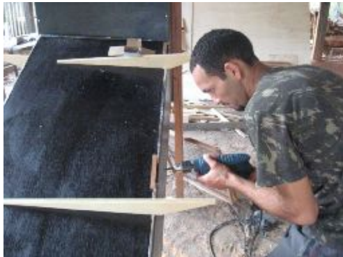
Figure 7.71: Fixing reflection sides to the dryer
