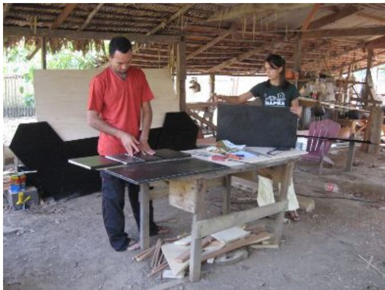
Figure 7.61: Working environment and sanding all parts of the dryer with abrasive paper
