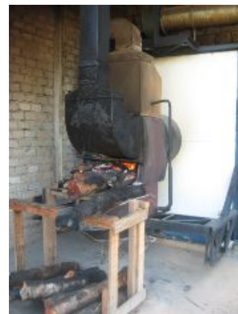
Figure 6.37: Energy supply for the dehydrator
