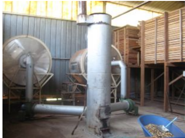
Figure 6.29: Dehydrator from the front with boxes for storage of nuts on the right side
